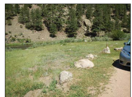
Photo 4 Boulders Used as Parking Limit
